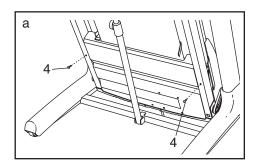
Lower the treadmill (see HOW TO LOWER THE TREADMILL FOR USE on page 25). Remove the four indicated 3/4" Screws (4), and remove the Hood (44).
